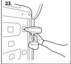
Open the clear polycarbonate cover by lifting upwards. Using a 7mm or 8mm masonry bit, drill through each of the 4 holes in the unit to make a small mark on the wall.
