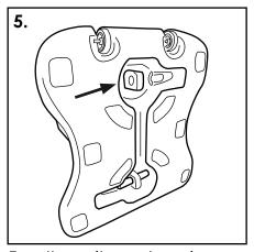
Turn the unit over to gain access to the other leg and repeat steps 3-4. The body and base are now secured together.
