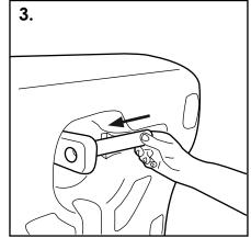
Taking one of the two pegs provided insert the rounded end first into one of the holes in the body leg.
