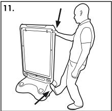
Place hand(s) around the side of the body and place your foot on the foot rest detail on the side of the base.
