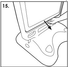
Place fingers into the opening recess at the bottom of the body and pull the clear polycarbonate protector away sides to secure it in position. from the body/magnets.
