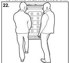
Lift the unit and position where suitable on the wall using a level to ensure it is horizontal. NOTE: the rectangular personalisation recess should be at the bottom.
