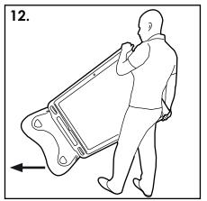
Using your foot and hands to lever the unit, tilt the unit towards you so that the wheels engage with the ground. Push the unit to its location.
