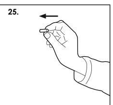
Insert a wall plug into each hole and lift the unit back into position on the wall.
