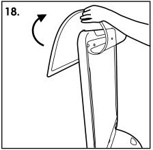
Unclip the clear protector from the press studs and pull back down into position over the poster ensuring all the magnets are connected.
