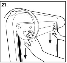
Pull the poster downwards from underneath the poster clips to remove. Unclip the clear protector from the press studs and pull back down into position over ensuring all the magnets are connected.
