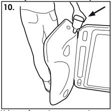
Using a funnel, pour sand through filler port until it reaches the level of the filler hole.
