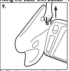
To fill with sand, lay the unit on its side in order to gain access to the fill port and remove filler cap.
