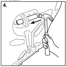
Using a hammer, tap the peg through the leg until it snaps in place (overrides lip) and locks.
