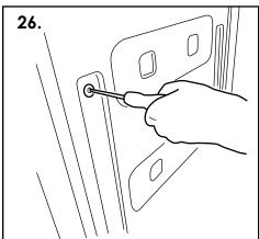
Place a 25mm washer onto a 60mm screw provided and push through hole in the unit. Place a 28mm spacer onto the screw so that is located between the unit and the wall. Locate the screw with the wall plug and fix the unit to the wall using a pozi drive screwdriver. Repeat on remaining 3 off fixing points. DO NOT overtighten.
