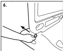
To fill with water, remove the filler cap on the side of the base. Ensure base is on a flat surface.
