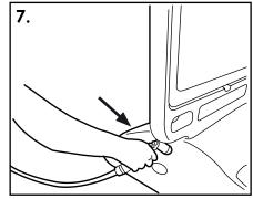
Using a hose fill the base until water reaches the filler hole. DO NOT over fill as there will be no space for expansion if the water freezes.
