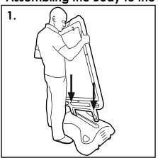
Place empty base on the ground and locate the two body legs into the slots within the base.
